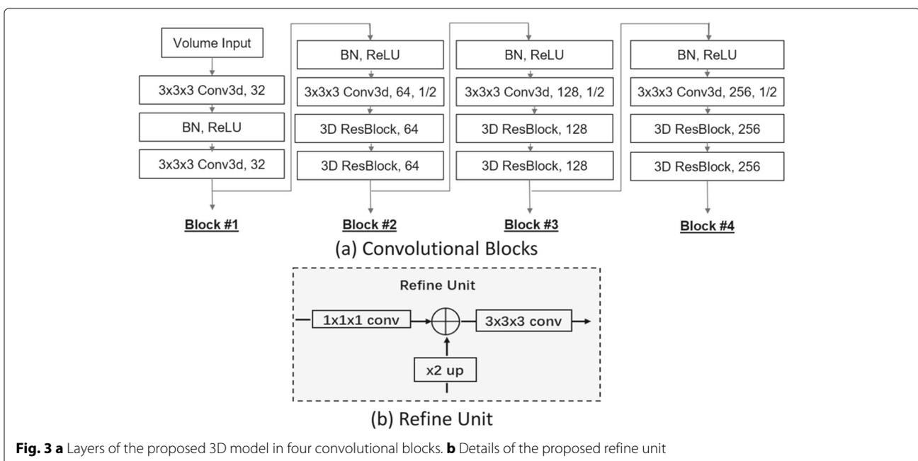
**Fig. 3 a** Layers of the proposed 3D model in four convolutional blocks. **b** Details of the proposed refine unit
