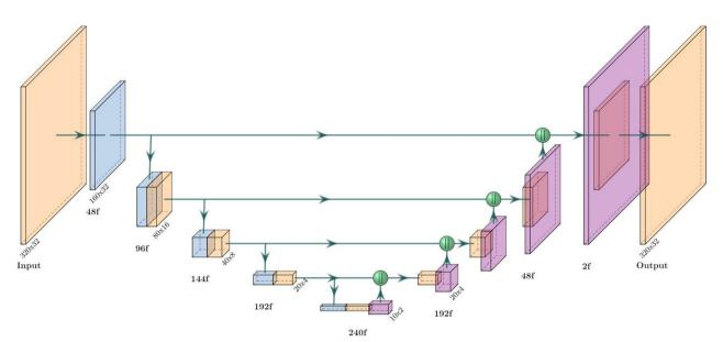
**Fig. 1** Architecture of our V-net segmentation network. Each block represents a residual convolution block (see Eq. 5); strided convolutions (downsampling) are blue and transposed convolutions (upsampling) are purple. The output resolution at each level is displayed and the number of filters/channels is displayed with the 'f' suffix. Green spheres represent concatenation. The last block performs 1x1x1 convolution with a sigmoid activation function
