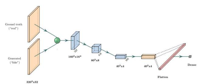
**Fig. 4** Architecture of the GAN discriminator. The ground truth and generated masks are first concatenated, then passed through consecutive strided convolution blocks (blue) and one regular convolution block. All blocks are non-residual Convolution blocks with  $4 \times 4 \times 4$  kernels followed by batch norm (apart from the first strided block) and a PReLU activation. The final dense layer uses a linear activation
