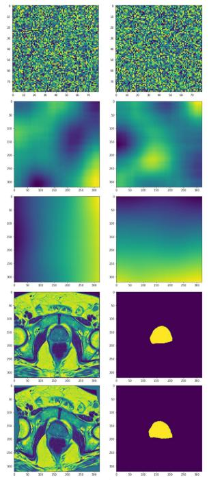
**Fig. 8** Visualization of the elastic deformation algorithm. The rows display *x* and *y* maps of steps 1-4 of the algorithm (top three rows), as well as the image and prostate mask of the original and the distorted image (last two rows)
