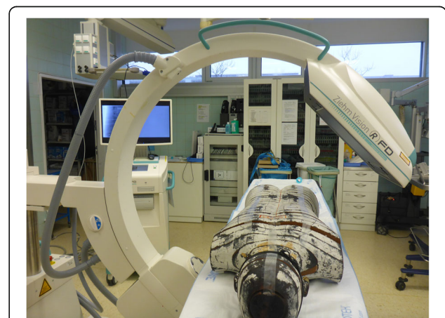
Fig. 1 An Alderson phantom was placed in prone position on a radiolucent operating table. The radiation exposure was measured at various sites (eye lenses, thyroid gland, female and male gonads) using dosimeters
